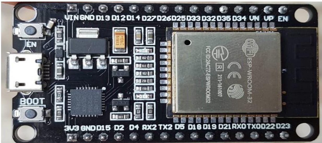
Figure 7: Espressif Systems 32 microcontroller board (Randomnerdtutorials, 2013)
