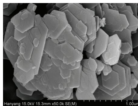
FIGURE 4: SEM micrograph of beneficiated kaolinite.
