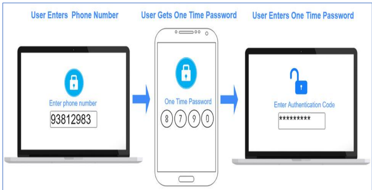
Figure 4: Two-Factor Authentication mechanism (Rahav, 2018)
