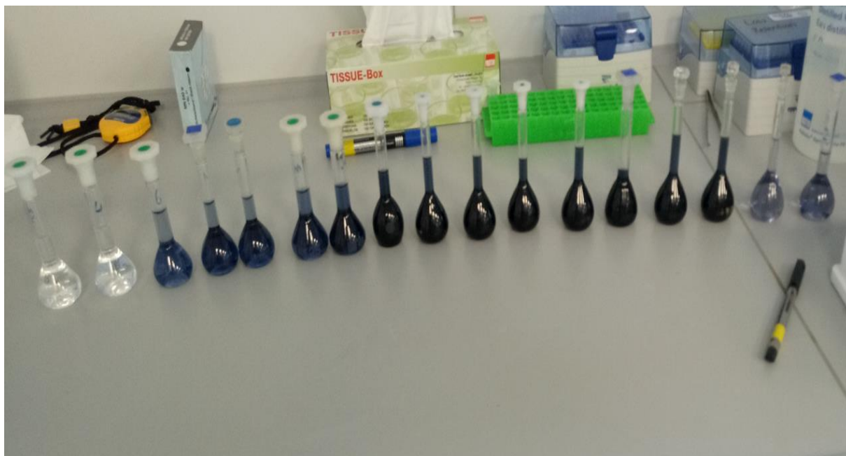
Figure 17: Samples for the Folin-Ciocalteu's assay to determine the Total Phenolic Content
