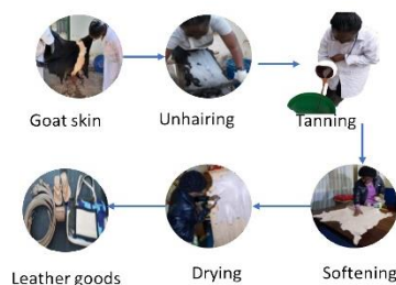
Figure 2: Scaling up of Goat skin processing using organic tanning chemicals to make leather
