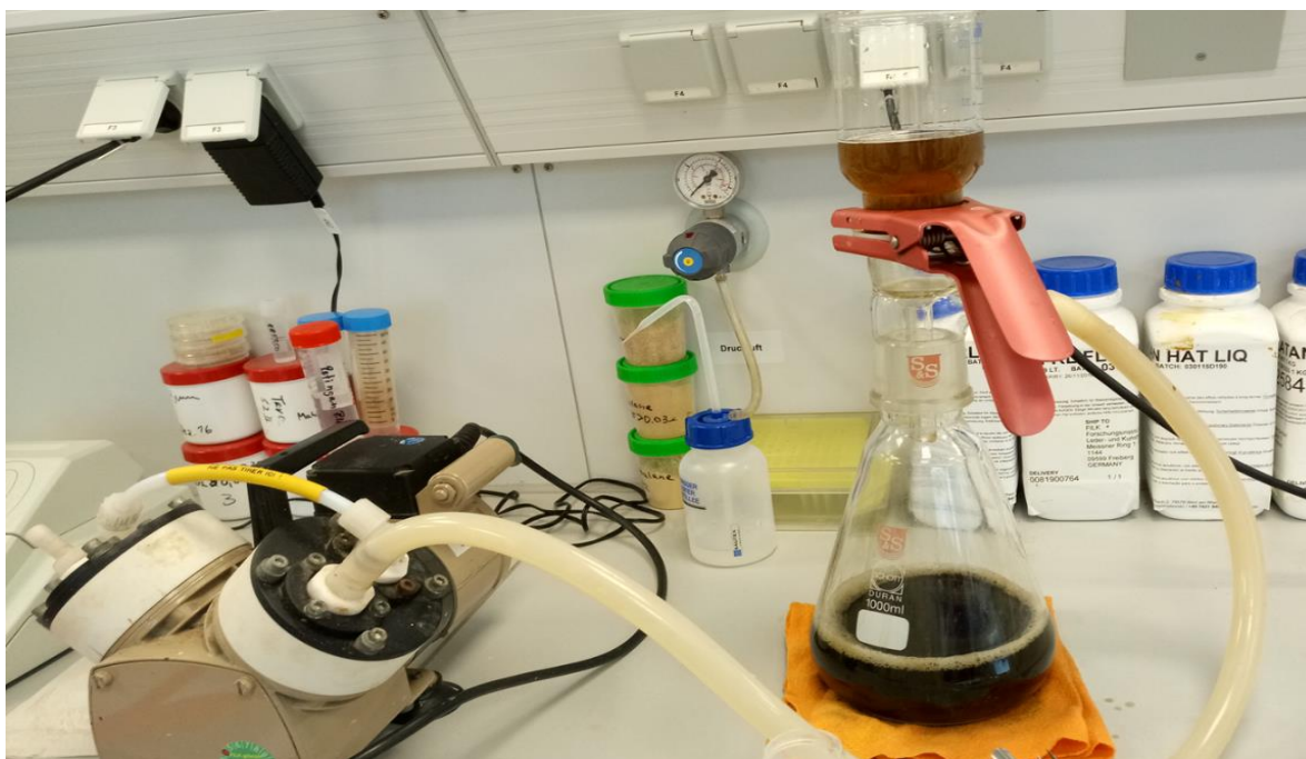
Figure 20: A vacuum pump filtering cross linked hide powder
