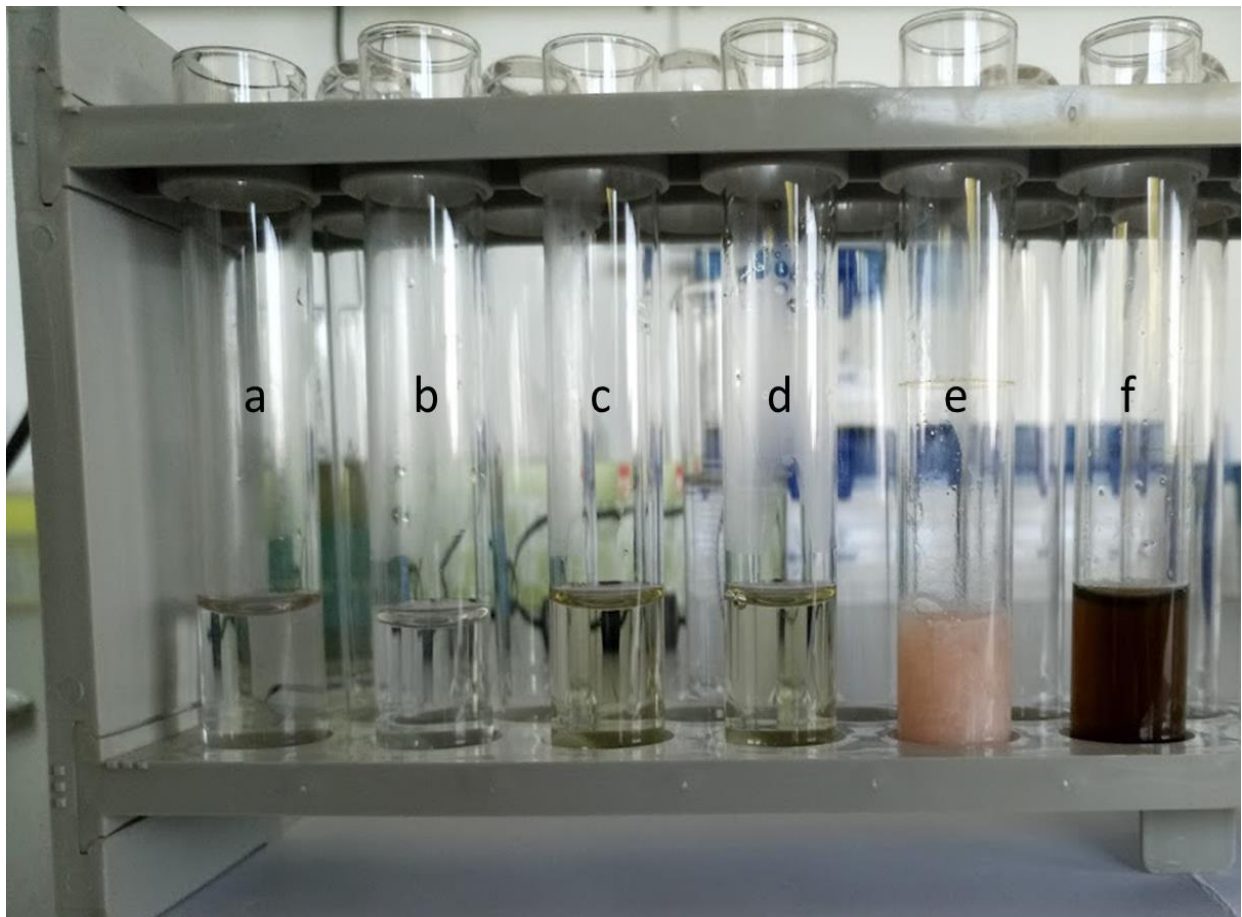
Figure 15: Gelatin test tubes. (a) water (b, c and d) detanned solutions of E. divinorum , A. mearnsii and A. xanthophloea , respectively (e) tannin solution (f) detanned solution of E. racemosa
