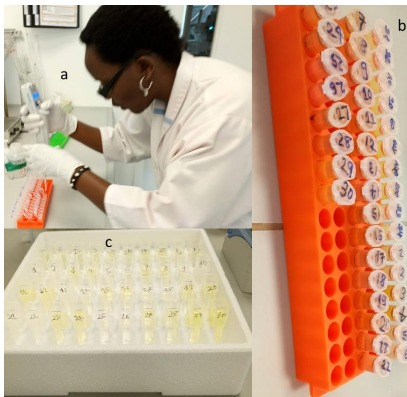
Figure 24: 2,4,6-Trinitrobenzenesulfonic acid assay (a) sample preparation (b) sample incubation (c) samples for measuring absorption
