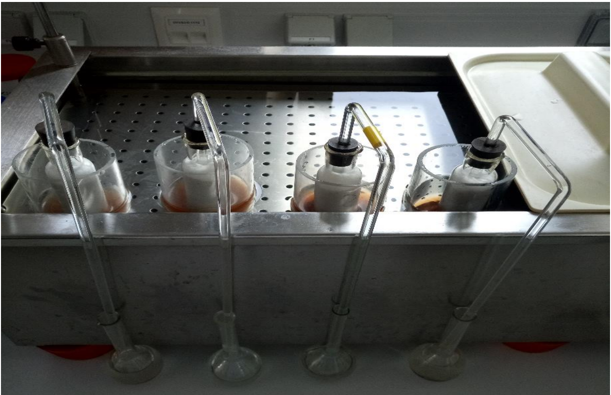
Figure 13: Experimental setup for the determination of tannin content
