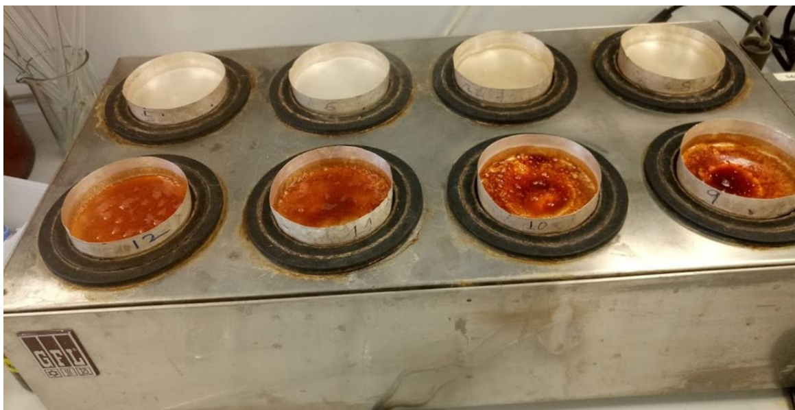
Figure 16: Evaporation of the detanned solution
