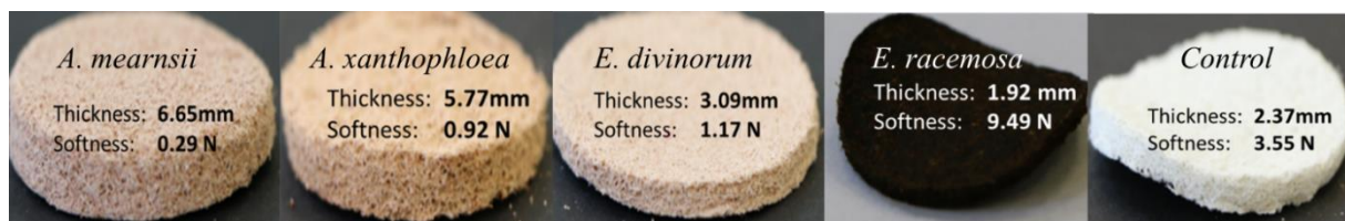
Figure 29: Hide powder tablets treated by the vegetable tannins from investigated plant barks
