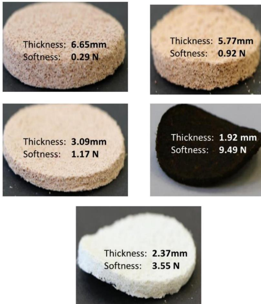
Fig. 4. Crosslinked and un-crosslinked hide powder tablets.
