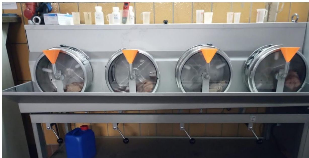
Figure 22: Tanning process in the experimental drums
