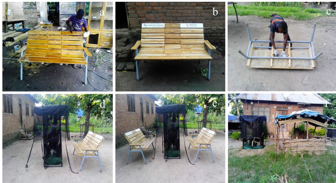
Fig. 2 Design and prototyping of the wooden chairs at the local carpentry (a), overview of the prototyped chair (b), fitting transfluthrin-treated hessian mat underneath the chair (c), one transfluthrin-treated chair with the DN-Mini trap positioned 0.5 m (d), two transfluthrin-treated chairs with DN-Mini trap installed 0.5 m (e); and outdoor kitchen fitted with transfluthrin-treated sisal ribbon with DM-Mini trap positioned 1.2 m (f)
