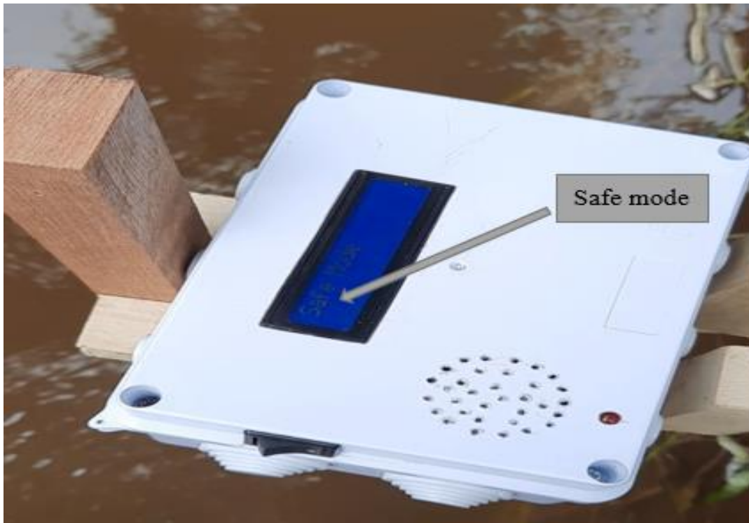
Figure 31: Display of the water level condition
