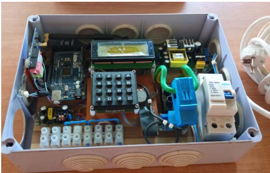
Fig.6. Smart Meter Unit Enclosed Inside a Water Proofing Box
