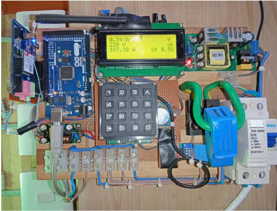
Fig.5. Smart Meter Unit During Testing
