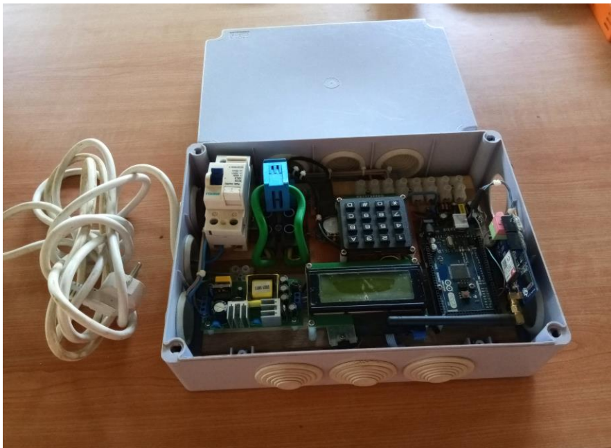
Figure 25: Smart meter unit enclosed inside a waterproofing box
