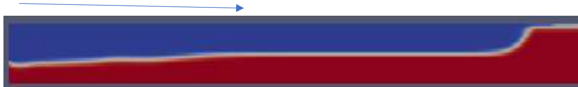
Figure 5: Liquid and Air Flows inside a Pipe for 1.0m Diameter at 3 degrees
