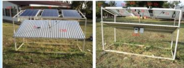
(a) Front view (b) Rear view Figure 2: Experimental setup: Three panels A, B, and C mounted on corrugated metal sheet (CMS) surface
