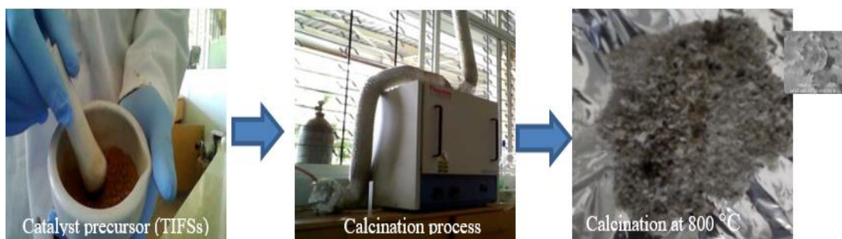
Scheme 3: Preparation and calcination process of TIFSA.
