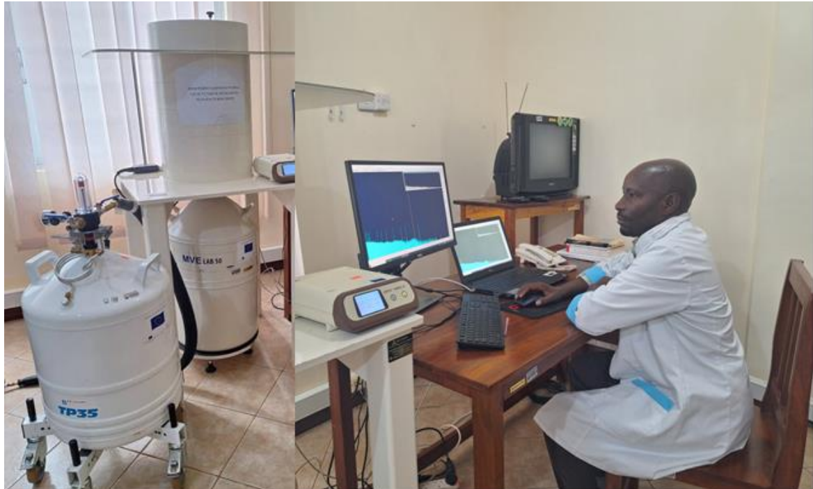
Plate 3: The HPGe Ortec Gamma ray Spectrometry System
