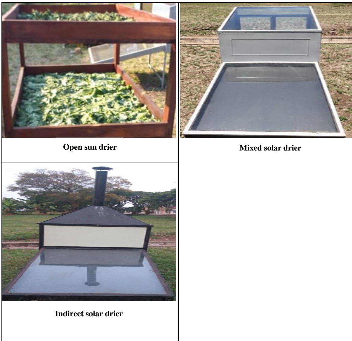
Plate 4: Different types of driers used in the study
