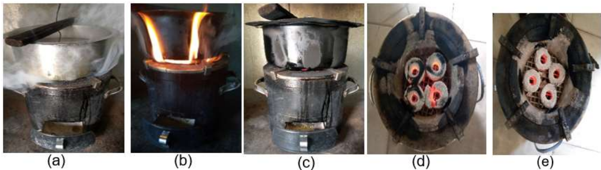
Figure 33: Combustion images; (a) Briquette B25 burning with white smoke, (b) Briquettes B25, B30, B35, and B40 burning with a yellow flame and soot (d) Briquettes burning without soot and yellow flame (e) Ash formation around the briquettes
