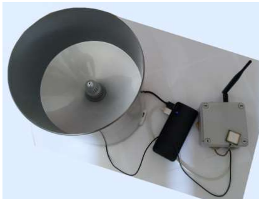
Figure 2: LoRaWAN end device
