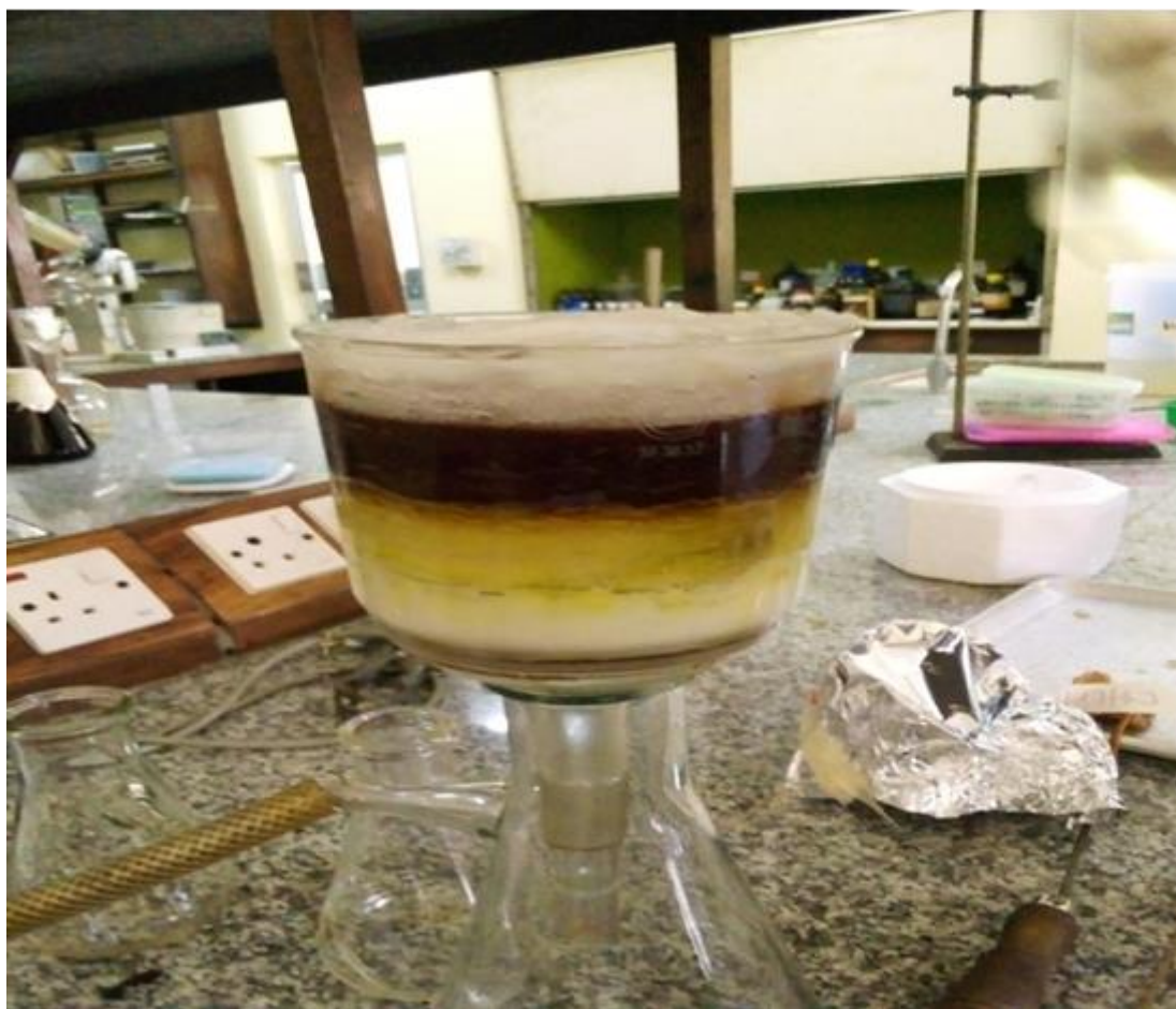
Figure 3: Shows the fractionation process, whereby DCM, EtOAc and Ethanol solvents were poured and then eluted using vacuum pump
