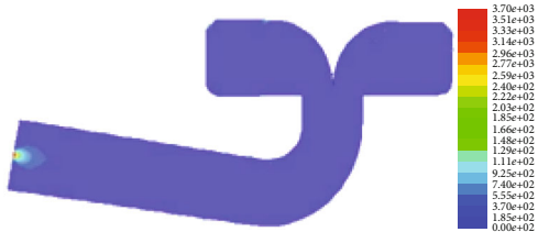
FIGURE 8: Contours of velocity distribution (m/s).
