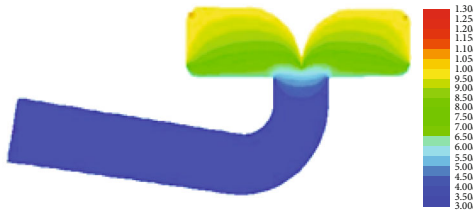
FIGURE 6: Contours of static temperature along the burner.
