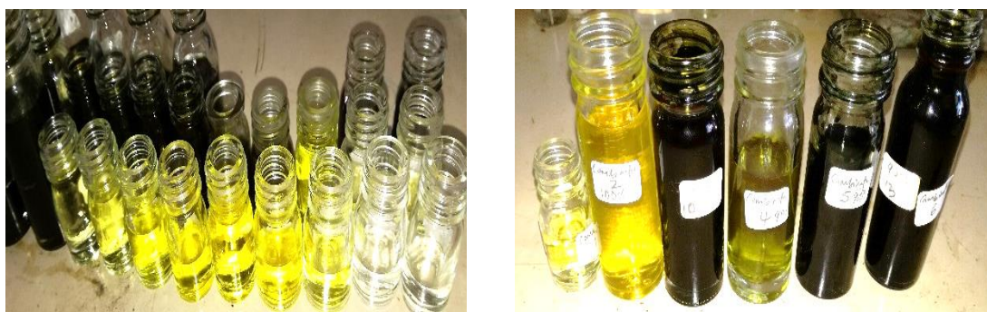
Figure 5: Fractions after column chromatography and fractions after combination as guided by TLC plates
