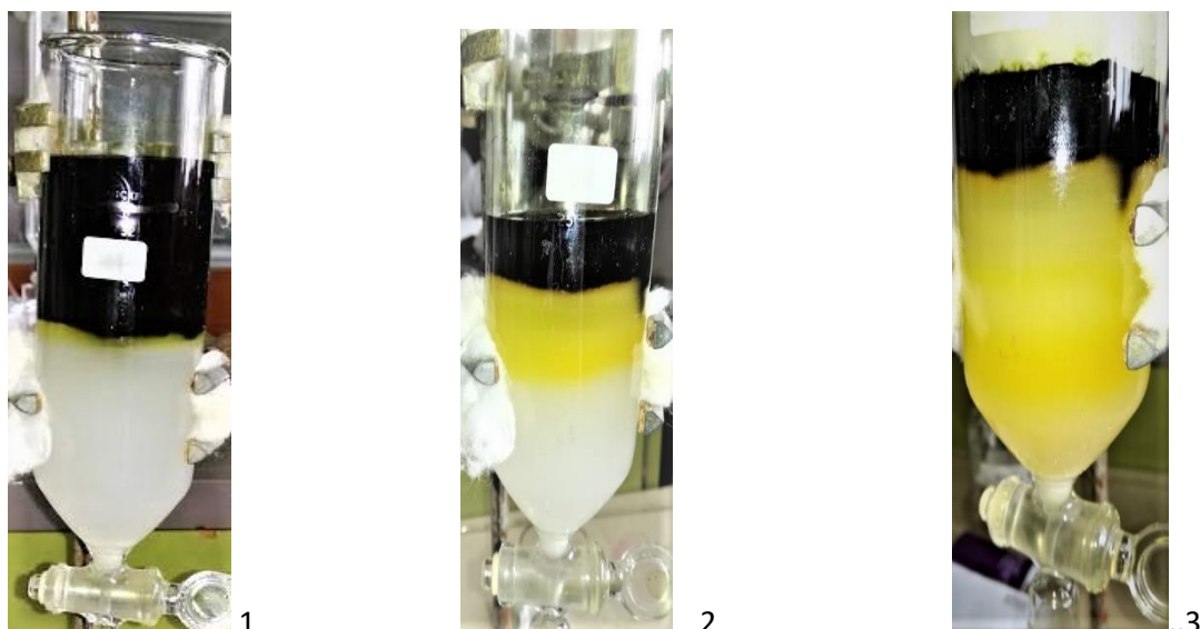
Figure 4: Liquid chromatography showing progressive development of fractions (1, 2 and 3 respectively)
