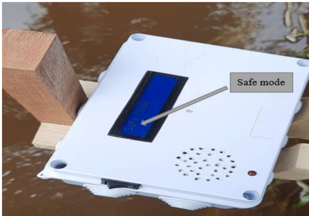
Figure 31: Display of the water level condition
